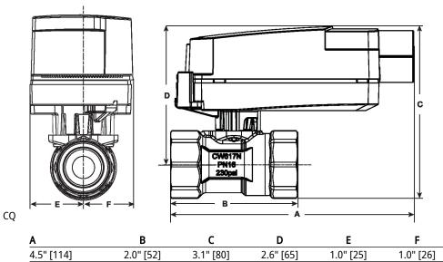
Modulating, Electrical fail-safe, 24 V
